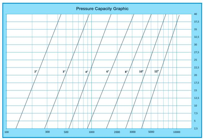
Maximum Flow Capacity (m<sup>3</sup>/h)
