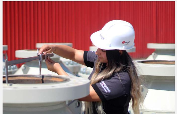
Fig.3. Storagetech™ Flame Arresters Control
